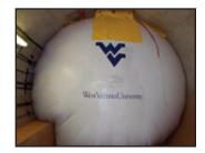
First RTC prototype for low inflation pressure
